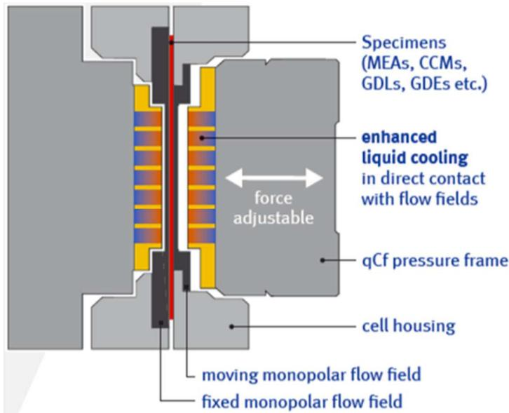
Figure 5: Design of Baltic cell unit
