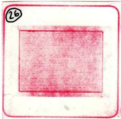
Figure 6: Even compression of the active cell area tested with pressure paper
