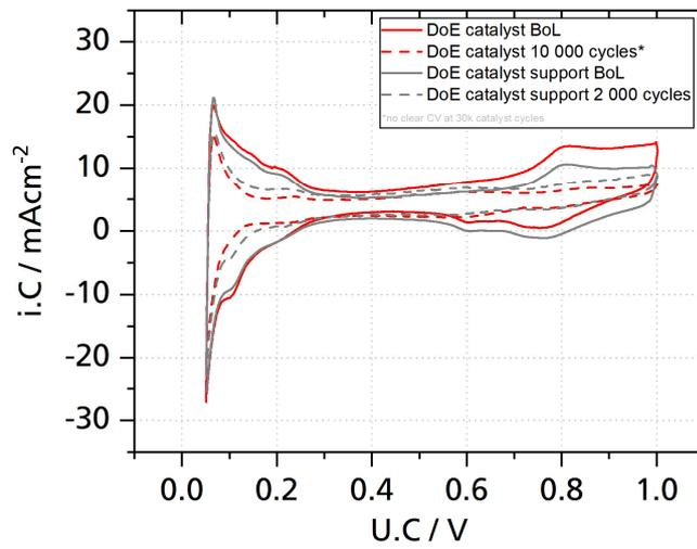
Figure 17: Cyclovoltammety BoL and EoT.
